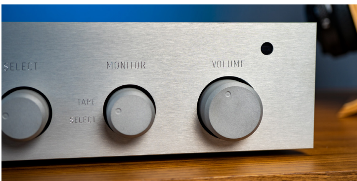
They still exist: The tape loop allows for tape monitoring when integrating a cassette deck or tape machine.
