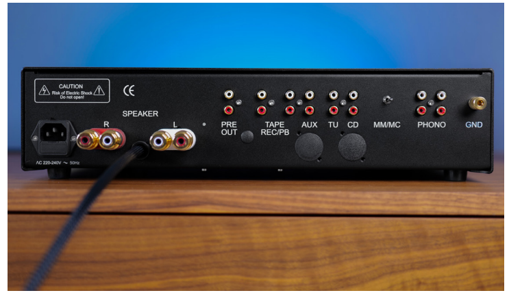
The entire rear panel of the RG 10 shows the ample analogue equipment of this amplifier
